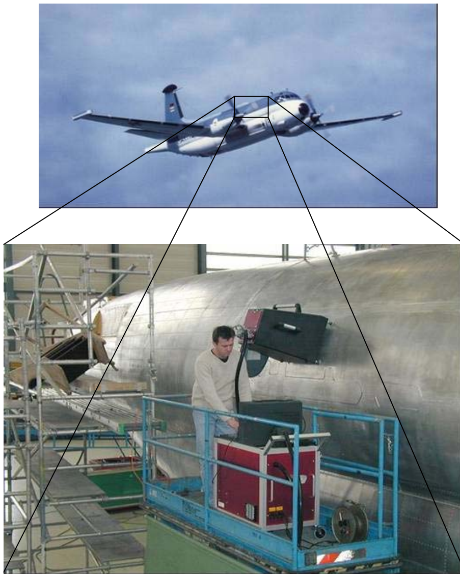
Figure 5: Mission Aircraft Breguet Atlantic (Detection of debondings in honeycomb structure).
