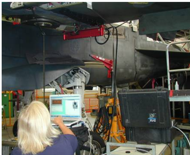
Figure 4: Fighter Aircraft TORNADO (Detection of corrosion at the wing diffusion joint).
